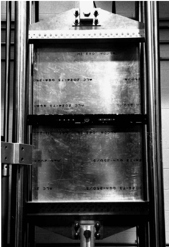
Photograph of actual test panel in the servohydraulic test machine
